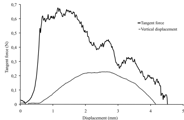
Fig. 6. Relationship between force of friction, T , and horizontal displacement, \Delta l , for pair of pea grains.
