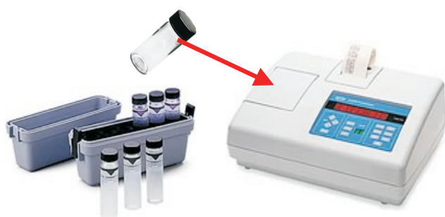
Fig. 2. Model HACH 2100 AN Turbidimeter as used for determination of the content of readily-dispersible clay, RDC .
