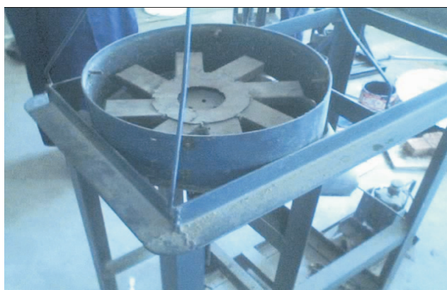
Fig. 4. Impeller mounted in operational position.
