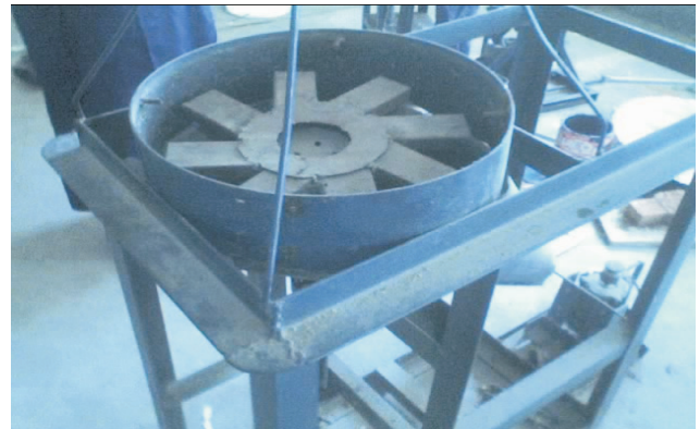
Fig. 4. Impeller mounted in the operational position.
