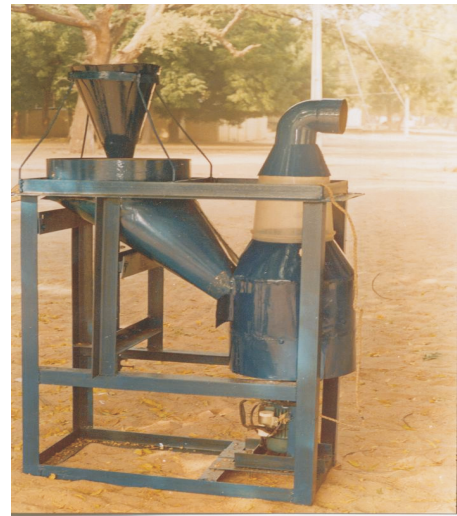
Fig. 1. Bambara groundnut sheller.
