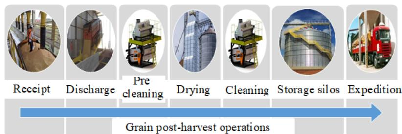
**Fig. 1.** General flowchart of seed pre-processing and storage operations.
