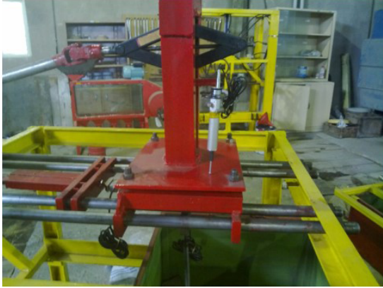
Fig. 3. Potentiometer mounted between the pressure plate arm and main plate on the rails.
