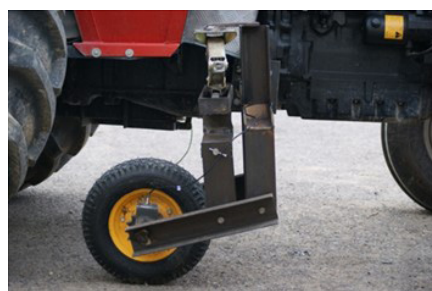
Fig. 2. Rreal speed measurement system of the tractor (fifth wheel).
